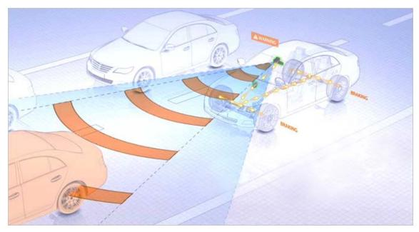
Automatic emergency braking made possible with sensor fusion technology
