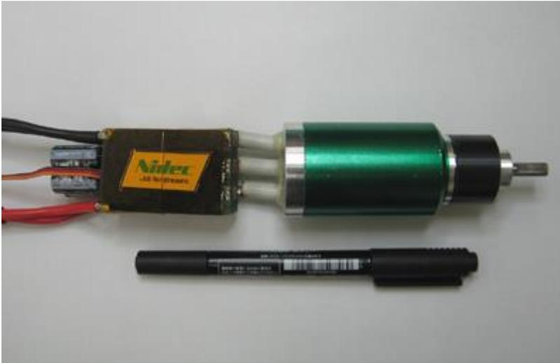
▲ F5B brushless motors and the Electronic Circuit Unit (ECU)
