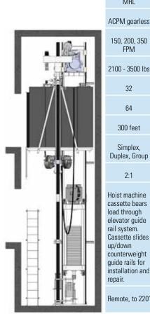
MRL ACPM gearless 150, 200, 350 FPM 2100 - 3500 lbs 32 64 300 feet Simplex. Duplex, Group 2.1 Hoist machine cassette bears load through elevator guide rail system. Cassette slides up/down counterweight guide rails for installation and repair.
