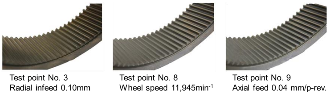
Fig. 11: Results of nital etching inspection
