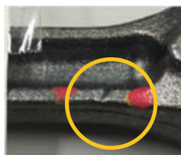
傷凹検出の例① Instance of concave defect ①
