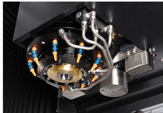
Blocks chips, grinding particles and coolant. The spindle nose section features a special anti-rust treatment and the ATC arm is coated in cold electric method.
