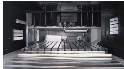
Covers enclosing the whole machine are provided as standard equipment to prevent chips and coolant from scattering and splashing outside the processing area. For protection of each slideway, scraper type stainless steel cover is provided on the X axis and bellows are on the Y and Z axes. All these features securely maintain the high machining accuracy.
