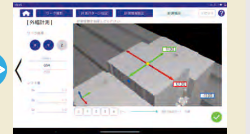
Automatic measurement for centering the workpiece
