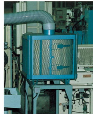
● Mist collector Equipment to recover oil mist produced during cutting
