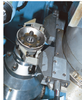
● Adjustable grip for part loader This grip can be quickly adjusted to accommodate parts of different diameters.
