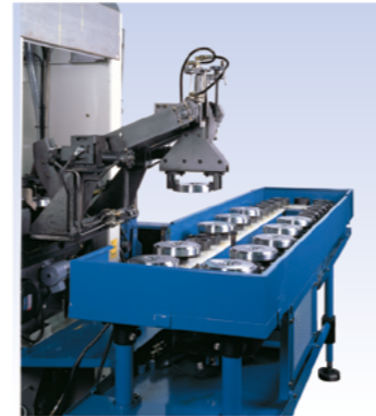
● Auto-loader, part stacker The combined use of the part stacker and transfer arm allows quick changeover of parts and is ideally suited for volume production.
