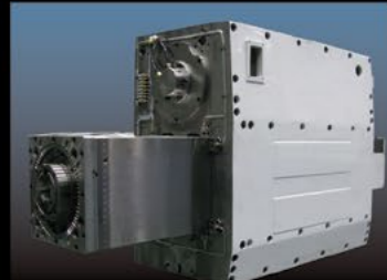
Ram: FCD600 (Ductile cast iron)
