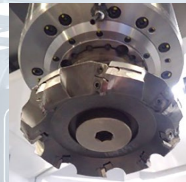
Material: S45C Tool Diameter: \phi 160mm \phi 6.3in Spindle Speed: 420min -1 Feedrate: 1,000mm/min 39.3ipm Cutting Depth: 5mm 0.20in
