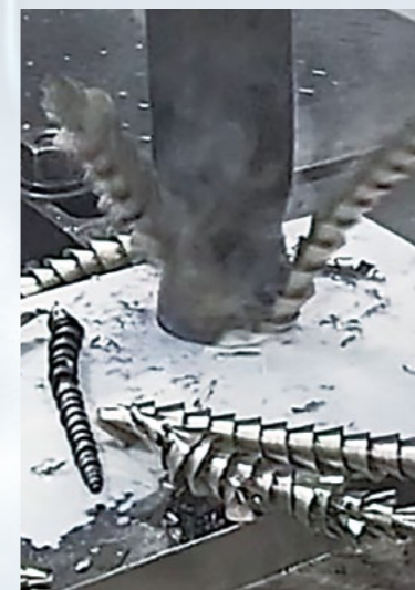
\phi 75mm \phi 2.95in Drill Material: S45C Spindle Speed: 90min -1 Feedrate: 30mm/min 1.18ipm
