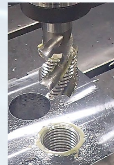
\phi 75mm \phi 2.95in Drill Material: S45C Spindle Speed: 90min -1 Feedrate: 30mm/min 1.18ipm
