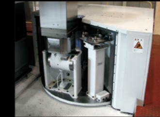
Equipping the right angle head
