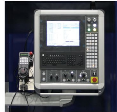
Operator Panel is movable and can come near the table for set-up.
