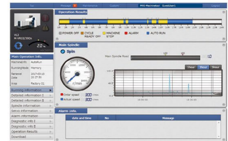
Confirmation Screen of Operation Monitoring
