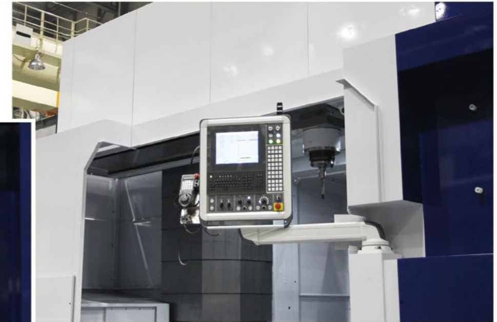
Operator Panel is movable and can come near the table for set-up.
