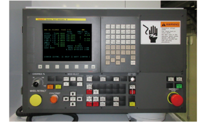
Operator's control panel
