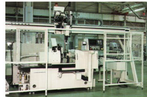
Gantry type two-gripper traveling auto-loader
