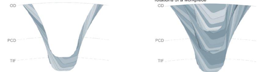
High circumferential feed means chips are removed thickly, so cutting teeth are distributed evenly, reducing wear.
