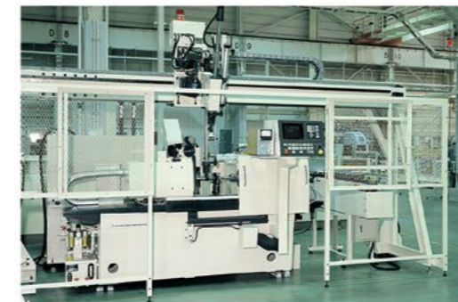
Gantry type two-gripper traveling auto-loader
