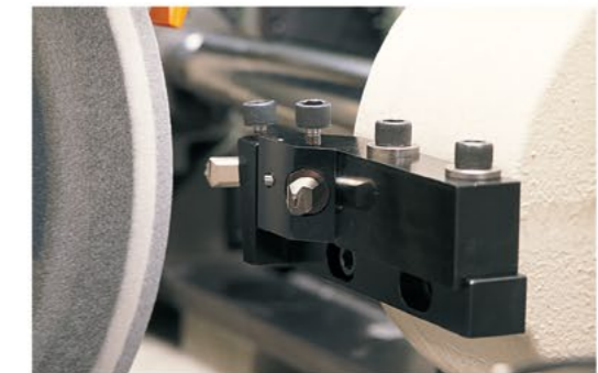
Two-head type single-point dresser holder
