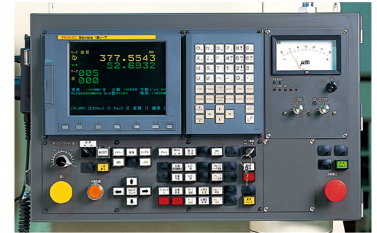
Operator's control panel
