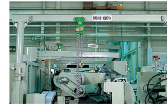
Jib crane for wheel change
