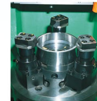
Three-cylinder clamping device
