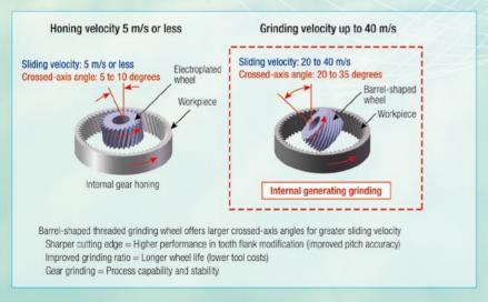
Generating grinding achieved by high-speed, high-precision synchronous rotation of wheel and work spindles
