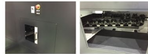
ATC Magazine door ATC Magazine Auto Tool Changer is located on the left side of the machine.
