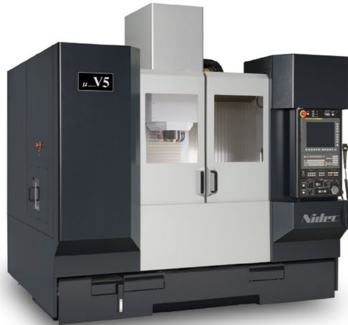
ATC Magazine door ATC Magazine Auto Tool Changer is located on the left side of the machine.
