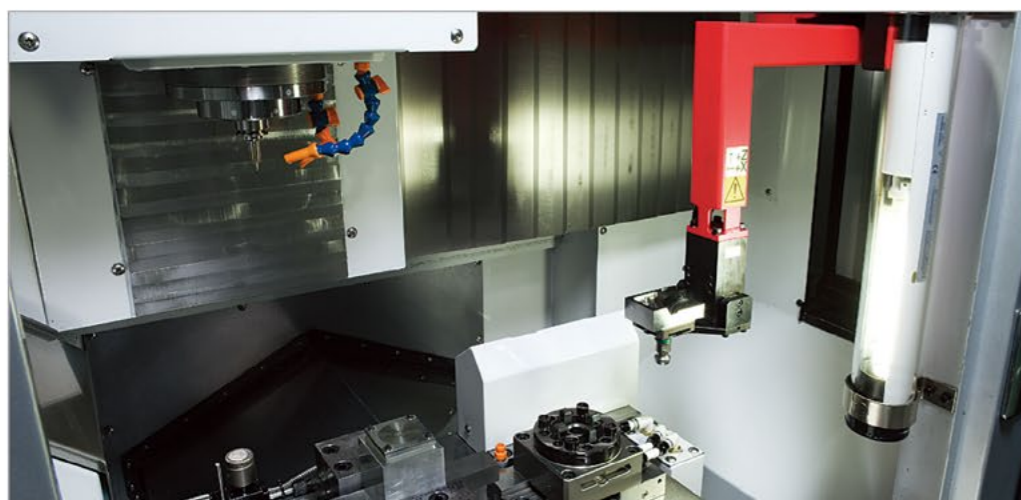
AWCワーク交換例(3軸仕様機) Workpiece change example using AWC (3-axis machine)
