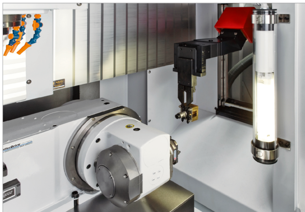
AWCワーク交換例 (5軸仕様機) Workpiece change example using AWC (5-axis machine)
