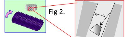
Fig 1. By set angle adjustment, Part tooth thickness decreases.
