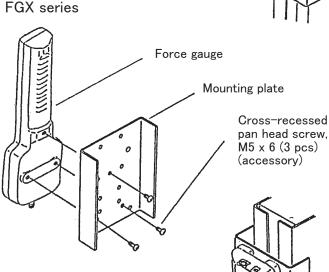
3) Mount the force gauge to the stand body by using the removed bolts.
