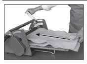
4.1. Turn the handle clockwise while guiding the board through the rollers in the direction of the arrow.
