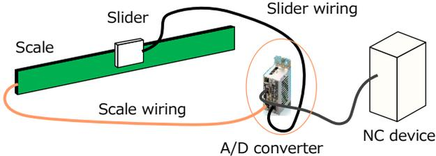
The electromagnetic induction method, the MPLW series' most prominent feature, possesses excellent durability that keeps detection accuracy from being affected by dust, oil, or condensation. Combined with other characteristics such as long and stable accuracy maintenance and thermal resistance based on a complete non-contact structure, this method is supported by various fields of industry.
