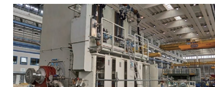
45MW hi-speed motor-generator
