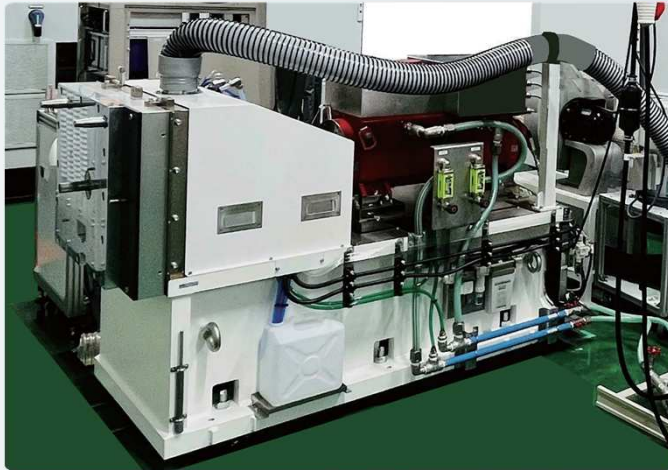
Example of System Configuration: Single-Axis Test Bench for EV Motors (20,000 rpm specification)
