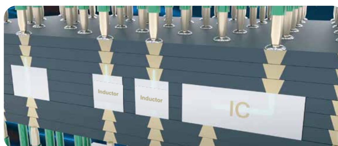
■ Low-Ls inspection of substrates embedded with SiC-MOSFETs and inductors
