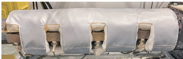
Injection molding machine with heat insulation cover attached
