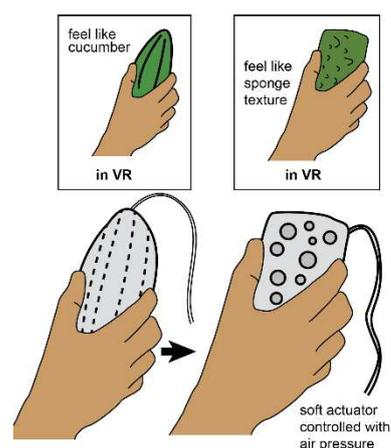
Figure 1 Proposed VR controller consists of soft actuators with programmable architectures.
