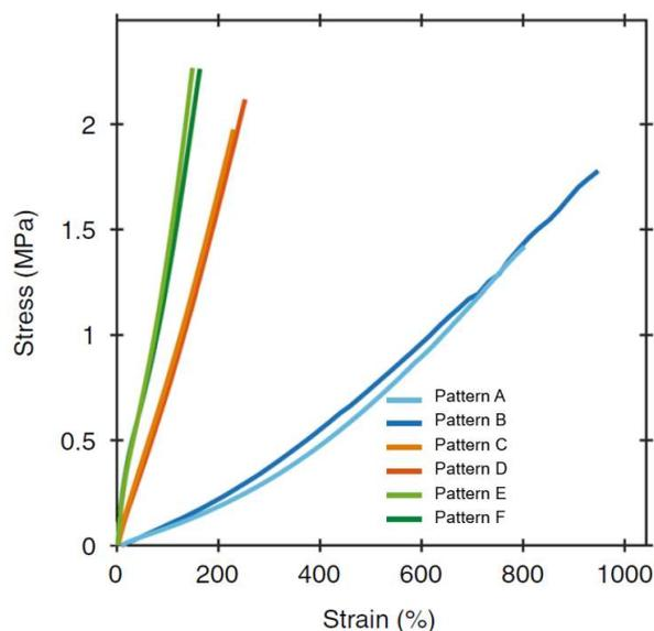
Figure 4 Mechanical behavior of printed soft actuator with different surface patterns.
