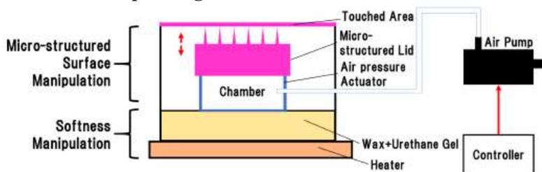
Figure 3 System diagram.
