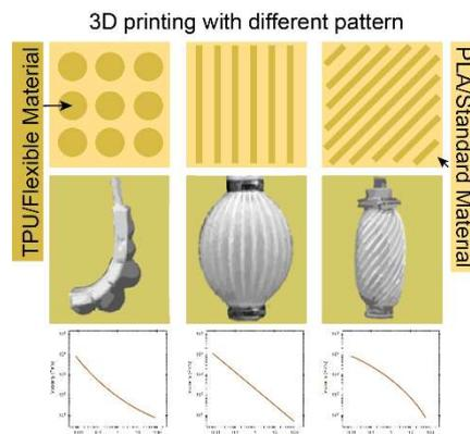
Figure 2 Illustration of 3D printed soft actuator with two materials (flexible and standard) hold the different shape characteristics depends on the printing pattern.
