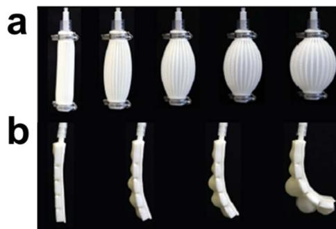
Figure 5 Soft actuator injected with hot air used in the experiment. (a) Horizontal line pattern, and (b) dot pattern.
