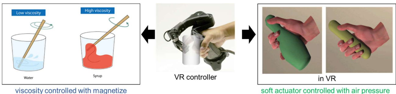
Figure 1 Proposed VR controller that can simulate the different viscosity perception (blue) in addition to the programmable soft actuator (green)
