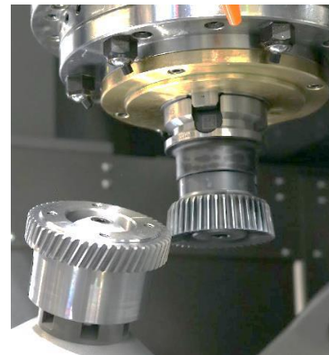
A gear-machining operation (example): A workpiece (left) and a cutter (right)
