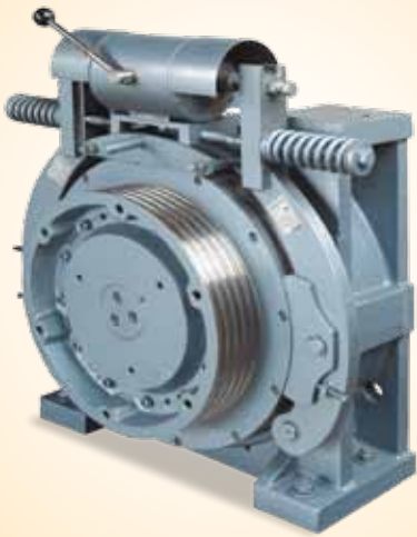
Frame 470 has the capacity to lift 1,375 to 4,000 lbs. at 100 to 500 fpm with 2:1 roping.
