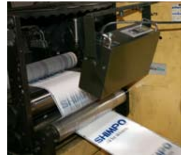
DT-329 Viewing Labeling Operation
