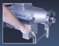
Access to mixing chamber for fast and easy clean-up
