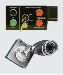
MCE's innovative MRL Remote Rescue<sup>™</sup> incorporates video imaging and battery power to allow a technician to safely move the car to a landing if commercial power is lost. A car-mounted camera sends video to an LCD screen in the controller. Using a button to control battery-provided brake lift power, and watching the LCD, the technician moves the car to a landing, aligning a marker on the LCD with a graphic in the hoistway to stop the car in the landing zone.
