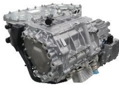
Ni150Ex (150 kW/3900 Nm) In mass-production since April, 2019
